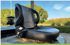
A full suspension seat that offers excellent comfort, with an operator safety system as standard.
