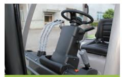
The instrument panel is fully sealed by covering parts, which is in accordance with requirements of European and American market.
