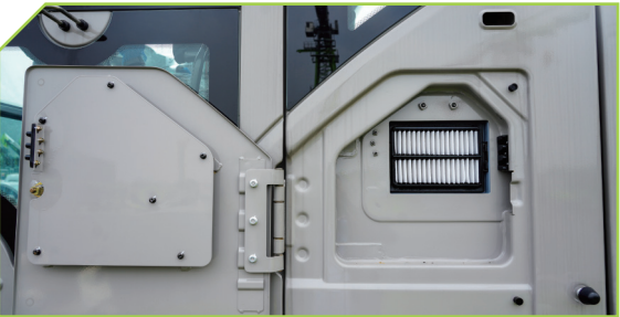
空调滤芯保养便捷 Convenient maintenance of air conditioning filter
