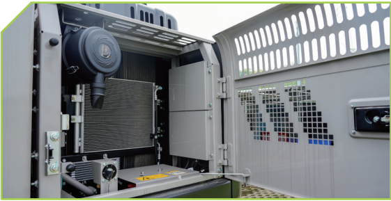
空滤保养伸手可及，玻璃水便捷加注，散热器集中式布置，加氟口加注方便 Air filter maintenance is within reach, glass water is easily refilled, radiators are centrally arranged, and fluorine filling ports are convenient for refilling
