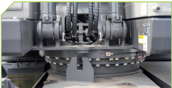
黄油集中润滑 Concentrated lubrication with grease
