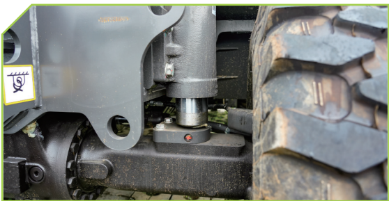
悬挂油缸垫板润滑，避免异响，防止过度磨损，提供舒适性和延长使用寿命 Lubrication of suspension cylinder pads to avoid abnormal noise, prevent excessive wear, provide comfort, and extend service life
