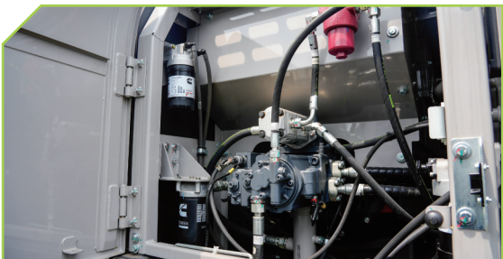
燃油滤、机油滤集中式布置 Centralized arrangement of fuel and engine oil filter
