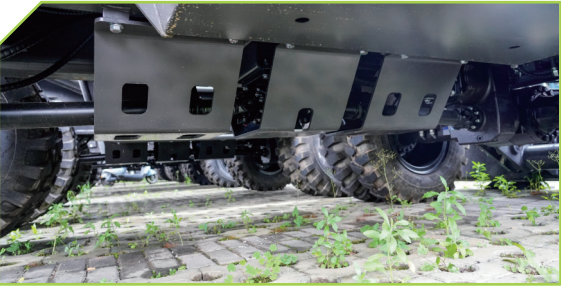
配备传动轴防护罩，有效避免传动轴磕碰损坏 Equipped with a protective cover for the transmission shaft, effectively avoiding damage and collision of the transmission shaft.
