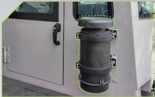
Pressurization system with effective external dust isolation
