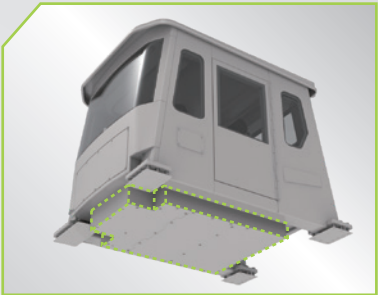
Cab protection in case of tire blowout: Featuring a bottom box-type structure, it will effectively protect the safety of driver.
