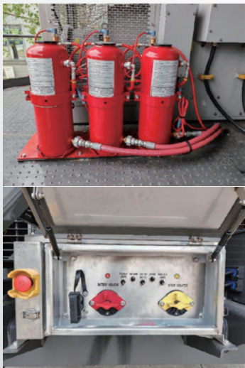
Rationally designed safety configurations: Full-automatic fire extinguishing system with 12 emergency stop buttons positioned across the fire suppression points on the machine
