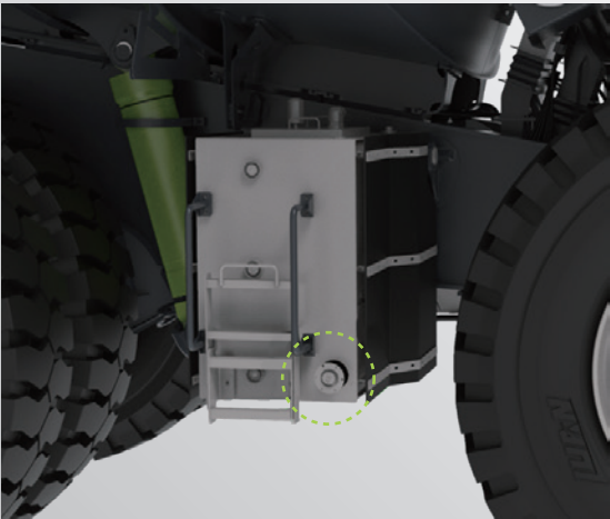
Fuel fillers are distributed on both sides of the frame, positioned close to the ground for quick refueling.
