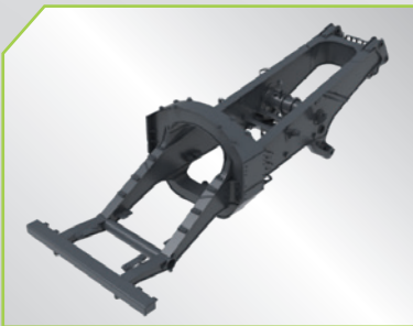
Two-longitudinal and four-transverse box-shaped welded frame: The main body is crafted from high-strength alloy steel, with cast steel applied to stress-concentrated areas, ensuring a designed service life exceeding 72,000 hours.
