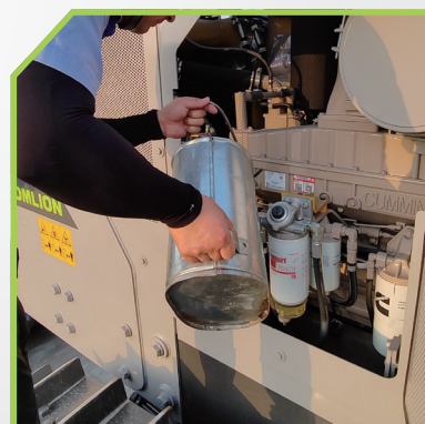
Refilling engine oil
