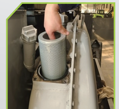
Hydraulic oil filter maintenance 液压油箱滤芯更换
