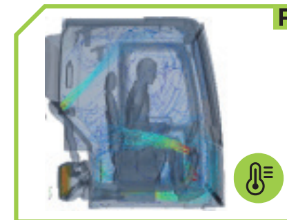
F Compared with the previous generation cab, the cooling effect of the new generation cab is increased by more than 19% 新一代驾驶室相比上一代驾驶室，制冷降温 效果提高19%以上
